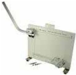
Here is a unique way to study horizontal and vertical motion, conservation of energy, and momentum. A track mounted to a vertical board directs one or two carts, casting them into a free fall. A brush projecting from the back side of the carts, marks the path of the cart as it falls. Weights can be added to the carts to study the effects of increased mass on momentum.
