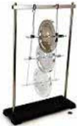
Used for demonstrating momentum, conservation of energy and torque. This unit which is basically a large flywheel is suspended by two strong cords. These cords are wound around the shaft of the wheel and then released. The wheel will unwind as it falls but will wind itself back up as the momentum carries the wheel upward in the opposite direction. This oscillation process will continue for several moments as the wheel slowly loses momentum and travels less each time.
