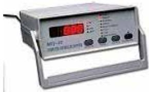
The solid state apparatus is a must for any physics class and is perfect for our air track and free fall apparatus. Two photo-gates are included, each with it's own shielded connecting cord and mounting screws. The timer has functions for timing, mechanical periods of oscillation, acceleration, collision velocities, counting and more.
