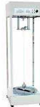
Measure the Earth's rotation in a smaller scale with this innovative instrument. A unique energy compensation mechanism enables continuous operation of the pendulum; glass windows shield the unit from drafts for uninterrupted, precision measurements; and a special 360° scale enables exact recording of directions. Designed for in depth analysis and advanced studies, this Foucault's Pendulum features amplitude adjustment and built-in illumination.
