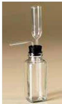
These gas generating bottles come complete with flint glass bottle, thistle tube, stopper and flint tube bent at 90 degree angle.
